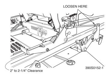
Figure 6-1. Brake Adjustment
